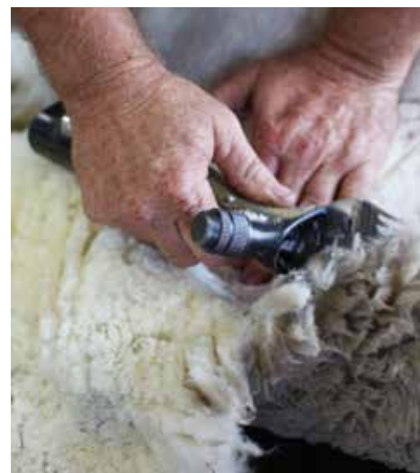
Shearing handpiece: Shearers use a specially-designed electric handpiece to remove the fleece.
