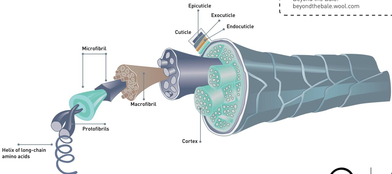
Structure of a wool fibre
