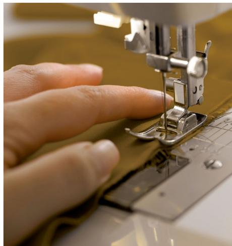
**Making up:** Woven fabrics are cut and sewn to produce garments ready for finishing.
