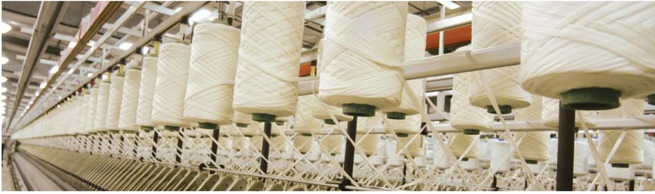
**Spinning:** Spinning machines insert twist into the woollen slubbings and worsted rovings to produce a yarn. These yarns can be woven or knitted to produce fabric.
