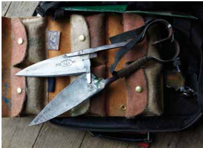
Blade shears: Shearers in the past used hand blades to shear sheep.
